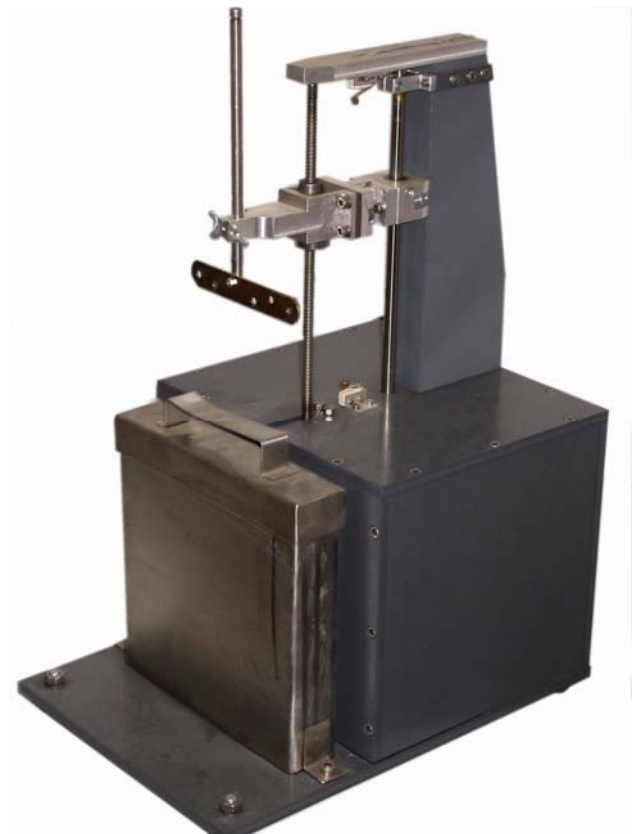
Fig. 10. System for photoresist coating of microwave substrate boards, designed by members of GIC. Reference [7].
