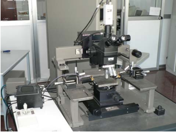
Fig. 7. CPW probe station on-wafer CASCADE MICROTECH Summit 10000.
