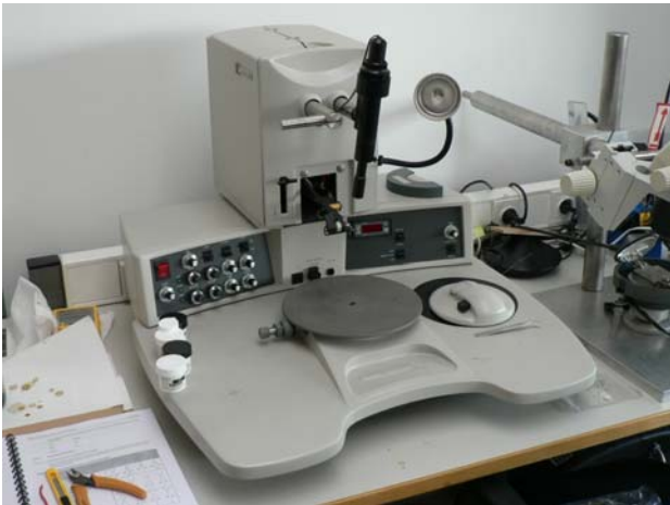
Fig. 8. Wire-bonding machine Kulicke and Soffa, model K&S-4523.
