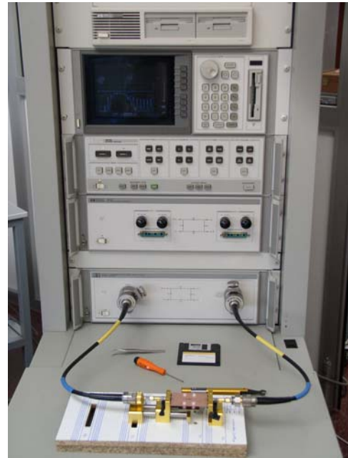
Fig. 9. Vector Network Analyzer Hewlett-Packard HP-8510B used to characterize devices.
