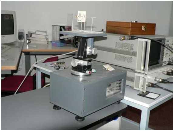
Fig. 11. Azimuthal positioner for a mm-wave band antenna test bench. Developed by GIC members.
